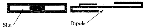
Figure 10a. The slot-dipole antenna, with ground and excitation. This shows the slot and the dipole, which are printed on one side of a flexible thin substrate.
